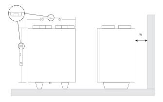
Horizontal floor-mounting positions on floor (W=400 mm)
