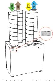
Figure. 2.3. Technical label place and air duct indication (right version)
