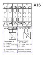
These sensors are intended for the following 3 functions: supply air pressure, extract air pressure and extract CO2 detection. Supply air pressure is measured inside the supply air duct referenced to the unit's surrounding area. Extract air pressure is measured inside the extract air duct referenced to the unit's surrounding area. The CO2 transmitter is installed in the extract air duct or room.
