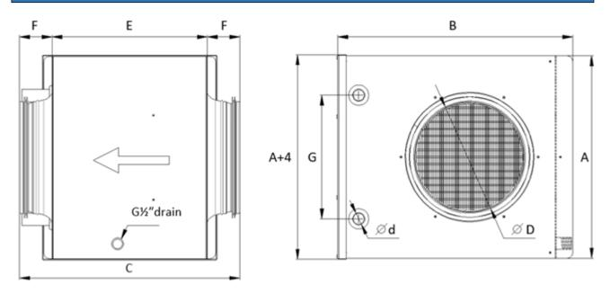
G½" drain is used in water coolers only.
