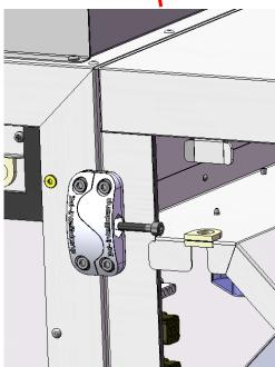
4. Screw condensate drain detail. The blue marked places grease with sealant.
