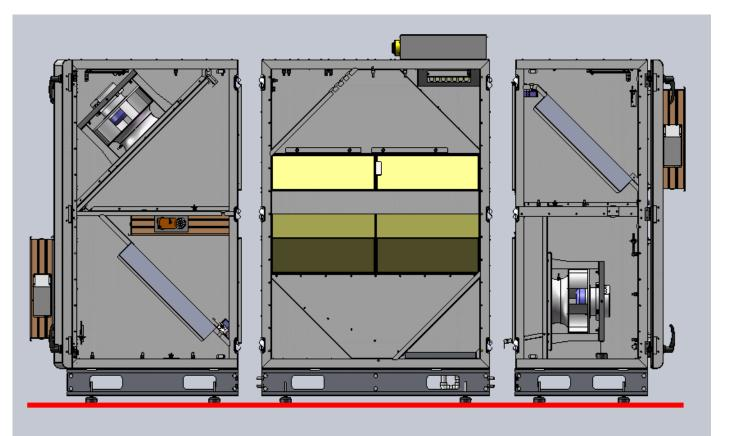
3. The sections are pushed together side by side, and connected with bolts.
