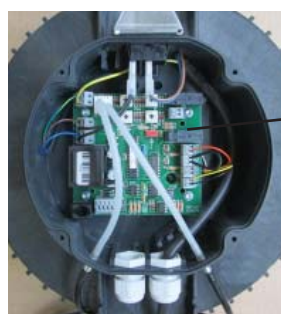
Fig. 4: Setting of differential pressure at the decade switches
