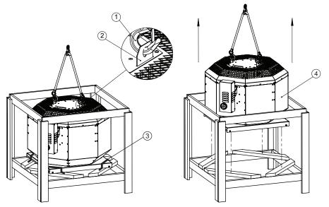
Lift the roof fan out of the packaging:
