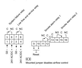
The relays are displayed in alarm mode, as they are in the event of a power outage.
