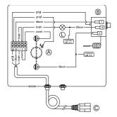
A= Heating coil B= Maximum safety with manual reset C= Connection plug 230V-50Hz L= Led maximum safety is activated
