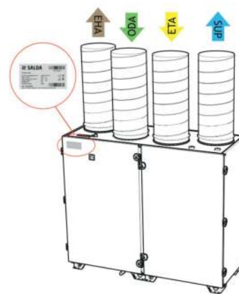
Fig. 3.3.6 Technical label place and air duct indication AmberAir Compact S-CX V (right version)
